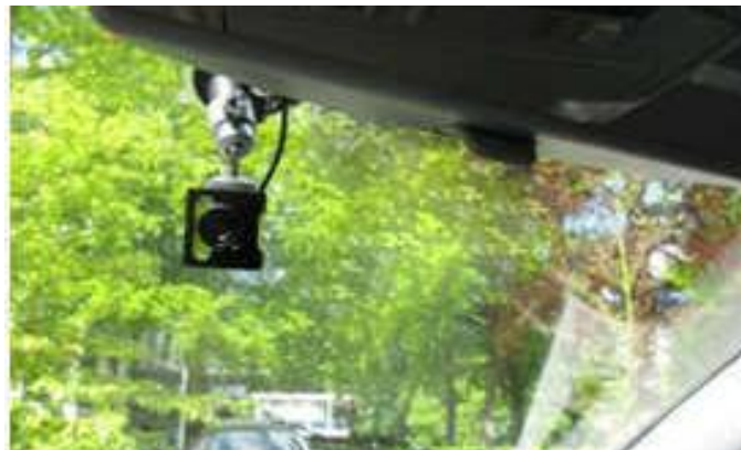
Figure 4: driver camera behind rear mirror
